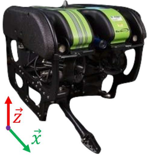
Fig. 2. A SeaBotix vLBV300 ROV similar to the one modeled in this work. Along with IMU and DVL sensors, the vehicle has six angled thrusters which control it along five degrees of freedom: heave (vertical z ), sway (lateral y ), surge (lateral x ), roll (rotation around x ), and yaw (rotation around z ).
